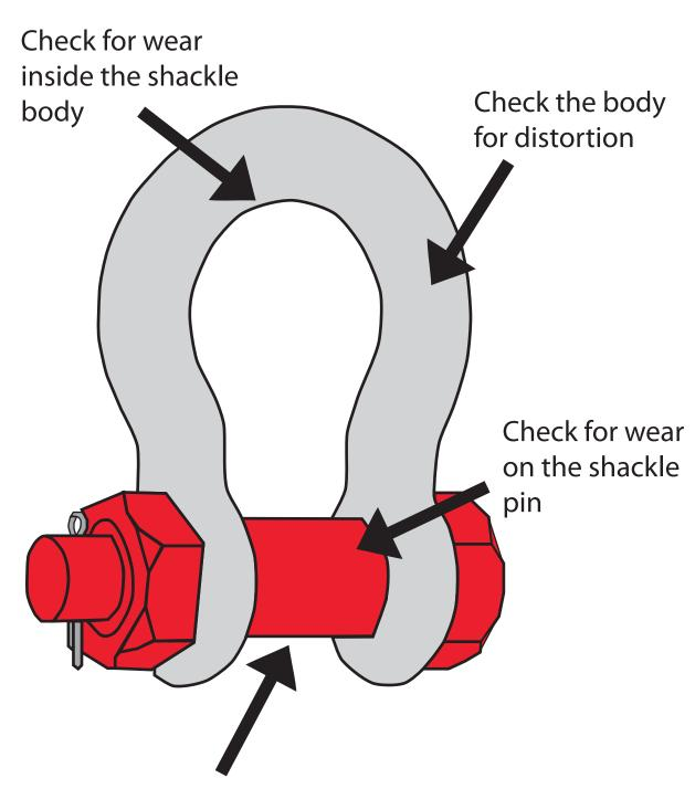
When a safety pin is used, ensure the plit pin is located correctly and secured
