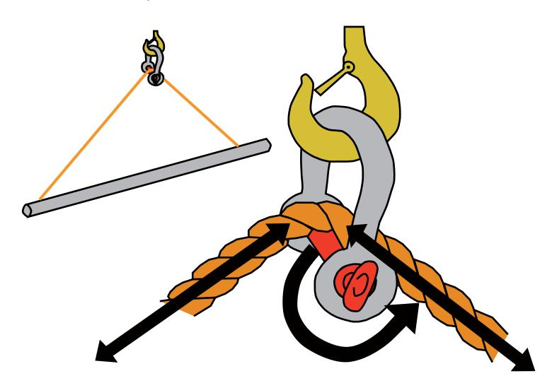
If the load shifts, the sling will unscrew the shackle pin.
