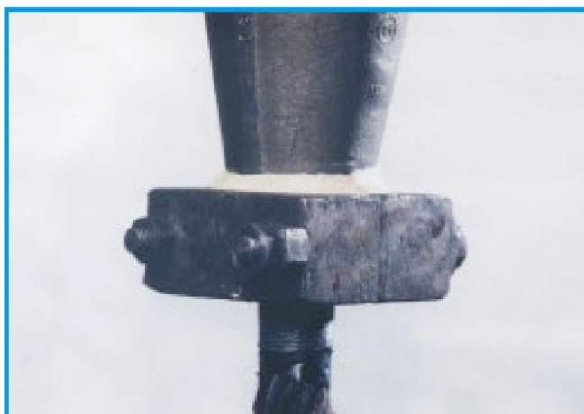
Clamp used to align rope and socket before sealing with plasticine (Fig 5)
