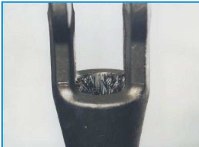
Properly positioned broom with the wire ends protruding slightly (Fig 3)
