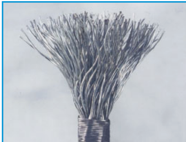
Properly Broomed Wire Rope (Fig 2)
